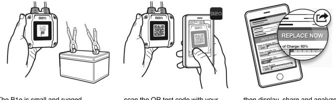
The B1e is small and rugged. Simply clamp it to a battery ... ... scan the QR test code with your mobile device running the free B2QScan app ... ... then display, share and analyze test results instantly!
